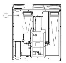
Fig. 5 Overheat protection reset button
